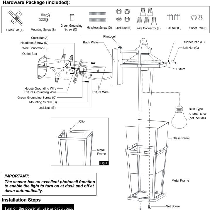
1. Thread two headless screws through the cross bar, and then secure them with four lock nuts (two on each side of the cross bar). Adjust the length of the headless screws if necessary.
