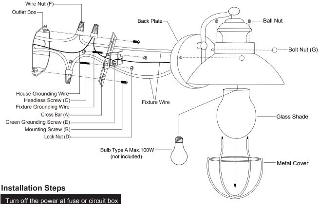
1. Thread two headless screws through the cross bar, and then secure them with four lock nuts (two on each side of the cross bar). Adjust the length of the headless screws if necessary.
